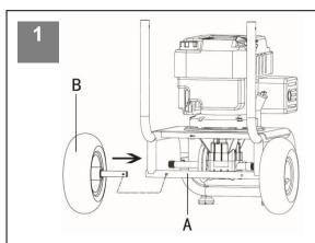
Lift the main frame (A) with one hand and attach one of the wheels (B) by pressing the wheel's pin and inserting the wheel shaft into the main frame (A). Align the pin with the hole on the frame (A) until it snaps in. Repeat this procedure for the second wheel (B) on the opposite side.
