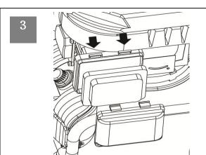
Press the two clips hard, and pull out the air filter element (12) and then wash it with clean water. Next, soak the filter in engine oil, and then squeeze the oil out. Place the air filter (5) back and re-clip the air filter cover.
