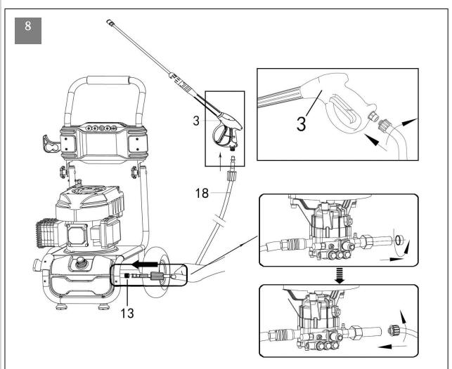
Attach one end of the pressure hose (18) to the spray gun (3) . Take down the air shield on pump water outlet (13), then attach to the other end of the pressure hose and fasten.
