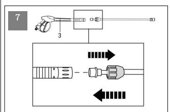
Assemble the spray gun with the metal wand (3). Pull back the rubber piece to expose the threaded fitting. Then, screw the two pieces together and move the rubber piece back.
