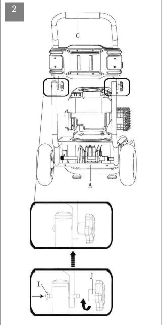
Position handle assembly (C) and main frame (A) as per instruction and connect them by square neck bolt (I), then secure by nut (J). Repeat this procedure for the second on the opposite side.BE SURE to secure the nut to make the handle upright.
