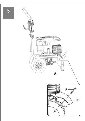
Insert the lower gun holder (F) to the position on frame as per instruction and then insert the bolt (K), screw the nut on the opposite position and secure by cross screwdriver (O) and wrench(Q)..
