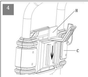
Insert hose hook (H) to the groove of handle assembly(C) until the end as per instruction.
