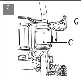
Insert upper gun holder (G) to the groove of handle assembly(C) until the end as per instruction.
