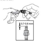
**NOTE:** In some areas, local law requires using a resistor spark plug to suppress ignition signals. If this engine was originally equipped with a resistor spark plug, use the same type for replacement.
