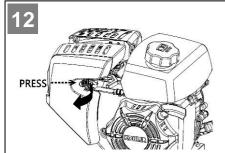
Press the right side of air cleaner housing and take it down. Take the air filter down and use water to clean. After cleaning, soak it into kerosene. Then put back the air filter to air cleaner, and fix the air cleaner housing.
