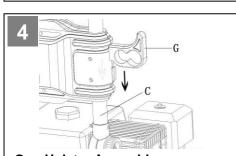
**Gun Holster Assembly**Attach the gun holster (G) to the frame side, slide down till in place.
