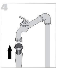
Attach garden hose to water supply and turn water on.
