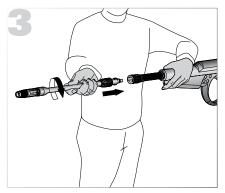
Insert the desired wand with nozzle into spray gun, and twist 1/4 turn until rectangular tab appears.
