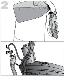
(when using detergent) Fill the detergent container with detergent and push lid firmly onto container. Attach detergent suction tube onto detergent lid and attach container to the pressure washer container storage area as shown.
