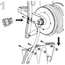
Insert handle frame into pressure washer and align the holes. Insert three nuts into the front, and insert the screws from behind as shown. Tighten the screws.
