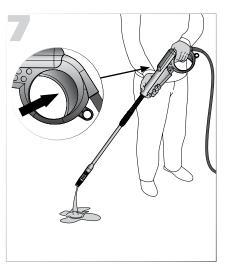
Purge air by squeezing trigger on the gun until there is a steady stream of water.
