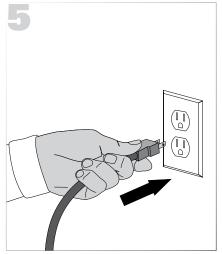
Make sure the main switch is in "OFF" position. Plug the unit into a properly grounded outlet.
