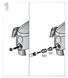
Remove and discard the cover. Separate quick-connect coupler assembly. Attach quick-connector coupler (M2) onto the garden hose and attach the inlet adaptor (M1) into the inlet.
