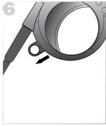
Release safety trigger, if locked.
