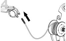
Assemble the high-pressure hose to the gun assembly.
