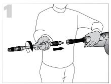
Install the adjustable wand. Set the adjustable nozzle to the low-pressure setting by sliding the nozzle collar out. The nozzle must be set in the low-pressure position to apply detergents.
