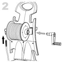
Attach the hand crank onto the hose reel. Assemble the extension hose to the reel.
