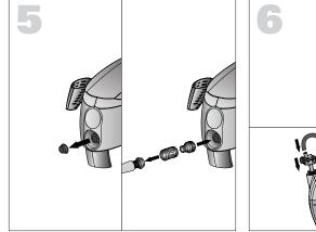
Remove and discard the cover. Separate quick-connect coupler assembly. Attach quick-connector coupler onto the garden hose and attach the inlet adaptor into the inlet.
