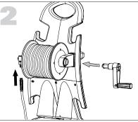
Attach hand cranks onto the hose/cord reel.
