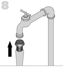
Attach garden hose to water supply and turn water on.
