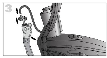
Gently pull detergent container out of storage position, and fill with detergent. Push containers back into storage position.
