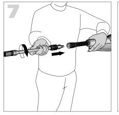
Insert the wand into spray gun and twist 1/4 to secure.
