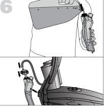
(When using detergent) Fill the detergent container with detergent and push lid firmly onto container. Attach detergent suction tube onto detergent lid and attach container to the pressure washer container storage area as shown.
