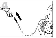
Attach high pressure hose from hose reel to the gun (hand tighten only).
