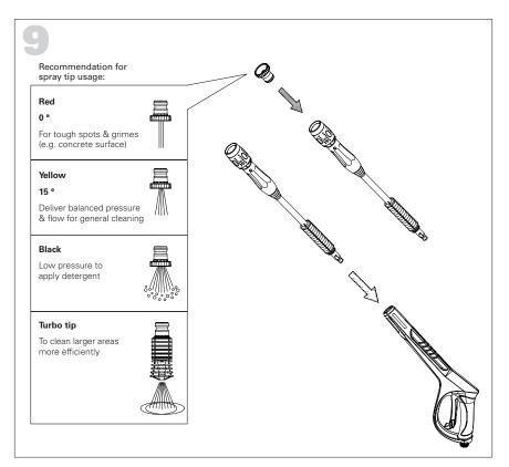
Attach desired coloured spray tip to wand. To install spray tips, gently slide the collar back before inserting the tip (see below).
