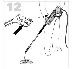
Purge air by squeezing trigger on the gun until there is a steady stream of water.
