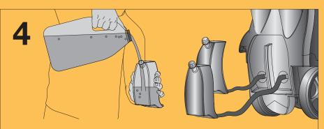
Fill two detergent containers and push lids firmly onto the containers. Attach detergent hose to the containers and push into the storage positions on the back of the pressure washer.
