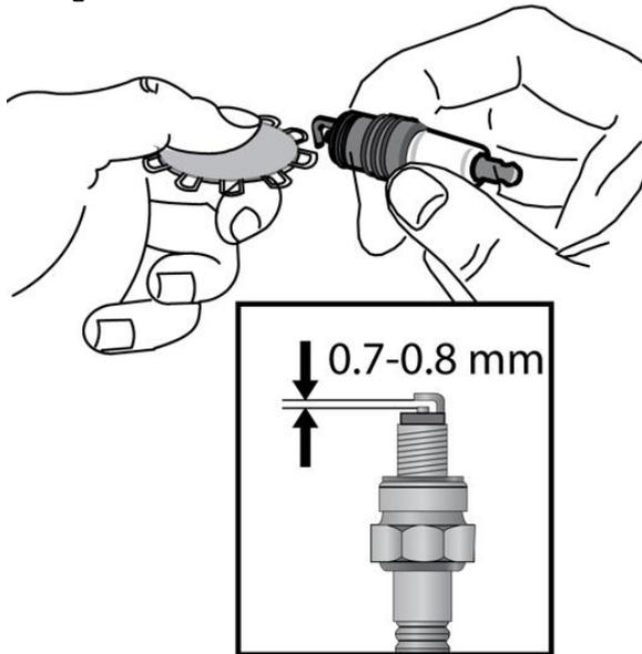
**Note:** In some areas, local law requires using a resistor spark plug to suppress ignition signals. If this engine was originally equipped with a resistor spark plug, use the same type for replacement.
