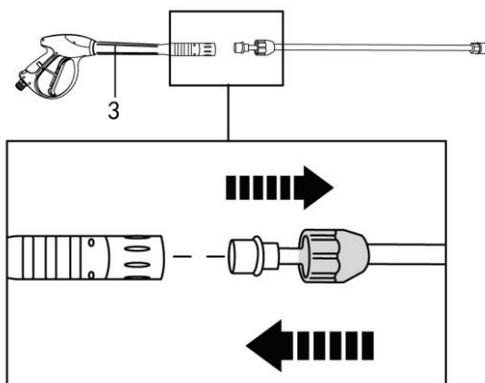
Assemble the spray gun with the metal wand (3). Pull back the rubber piece to expose the threaded fitting. Then, screw the two pieces together and move the rubber piece back.
