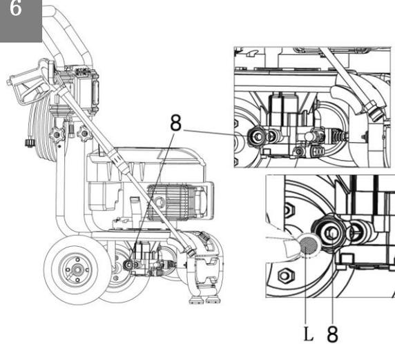
Insert the water inlet filter (L) into the pump fresh water inlet (8). Then attach a garden hose or other means of water supply (not provided) to the pump inlet (8).
