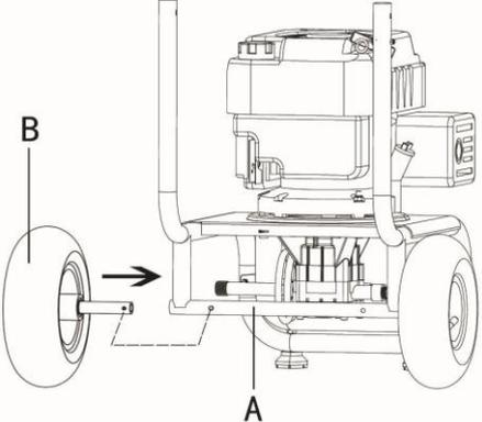
Lift the main frame (A) with one hand and attach one of the wheels (B) by pressing the wheel's pin and inserting the wheel shaft into the main frame (A). Align the pin with the hole on the frame (A) until it snaps in. Repeat this procedure for the second wheel (B) on the opposite side.
