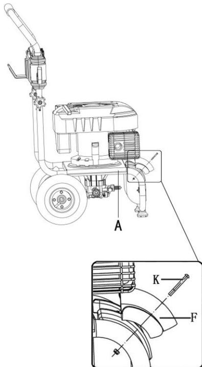
Insert the lower gun holder (F) to the position on frame as per instruction and then insert the bolt (K), screw the nut on the opposite position and secure by cross screwdriver (O) and wrench(Q)..
