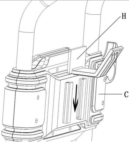
Insert hose hook (H) to the groove of handle assembly(C) until the end as per instruction.
