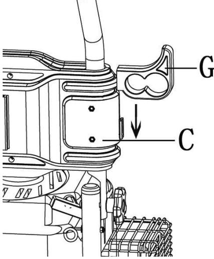
Insert upper gun holder (G) to the groove of handle assembly (C) until the end as per instruction.
