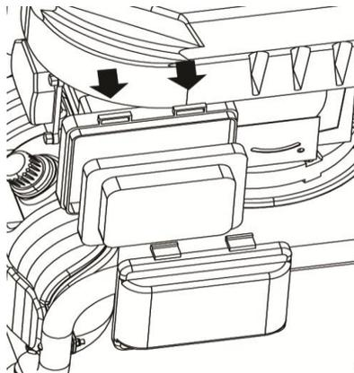
Press the two clips hard, and pull out the air filter element (12) and then wash it with clean water. Next, soak the filter in engine oil, and then squeeze the oil out. Place the air filter (5) back and re-clip the air filter cover.
