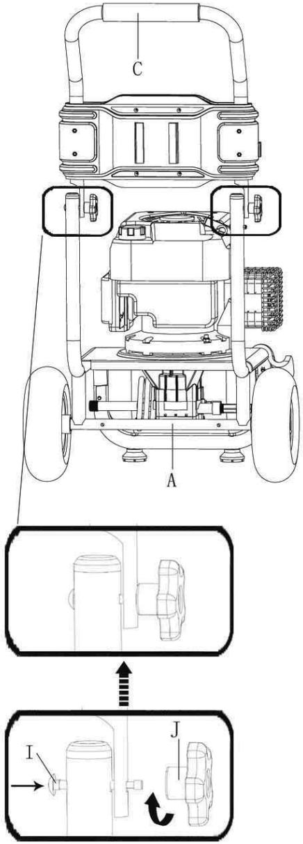
Position handle assembly (C) and main frame (A) as per instruction and connect them by square neck bolt (I), then secure by nut (J). Repeat this procedure for the second on the opposite side. BE SURE to secure the nut to make the handle upright.
