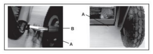
2. Install the panel to top handel, then install the top handle to the frame by sliding the top handle posts into the frame posts and secure them together using 2 pan head bolts, 4 washers and 2 nylon hex nuts.
