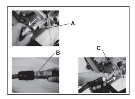
6. Assemble the stainless steel wand (A) and the metal gun(B). Pull back the rubber piece(C) to expose the threaded fitting and screw the 2 pieces together, re-position the rubber piece.
