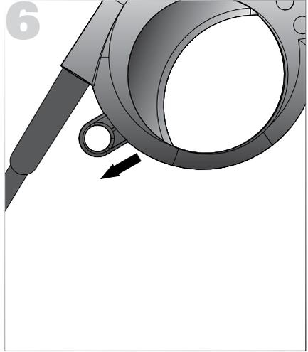
Release safety trigger, if locked.
