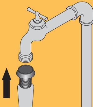
Attach garden hose to water supply and turn water on.
