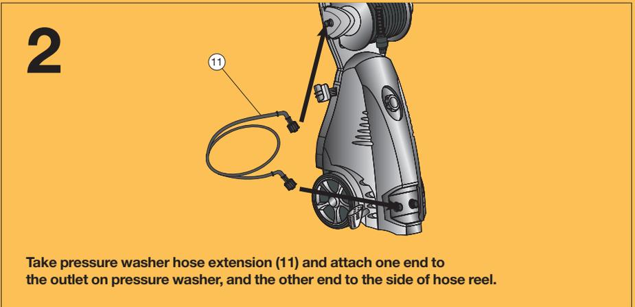
Take pressure washer hose extension (11) and attach one end to the outlet on pressure washer, and the other end to the side of hose reel.
