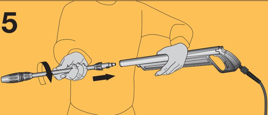
Insert the desired wand into spray gun and twist. Turn until rectangular tab appears.
