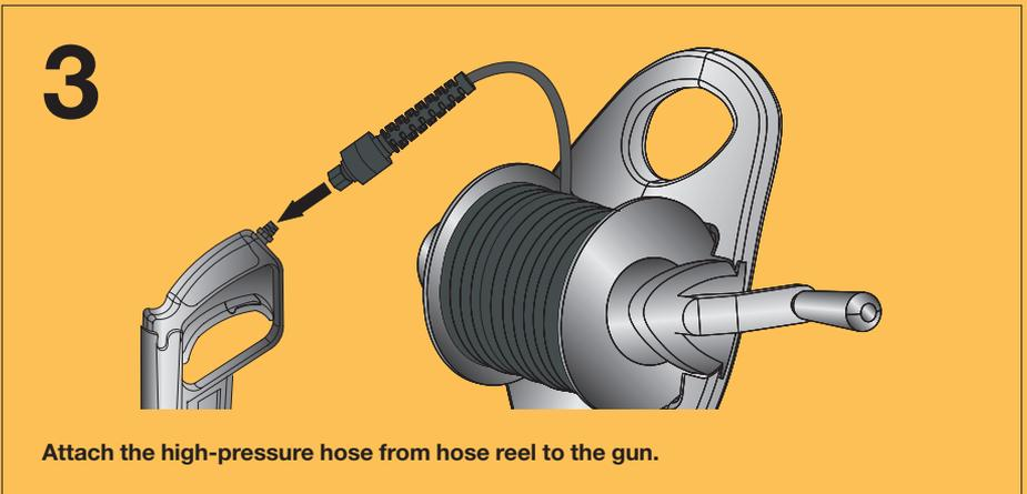
Attach the high-pressure hose from hose reel to the gun.
