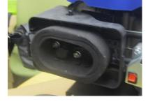
**If Washing Filter:** Wash dirty Air Filter with high-flashpoint solvent such as mineral spirits or paint thinner. Squeeze gently to dry and avoid twisting or tearing the Filter. Lastly, dip in clean engine oil, squeeze out excess oil.
