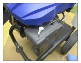
STEP 1: The Carburetor is located behind the Air Filter. Remove the Air Filter to access the Carburetor.
