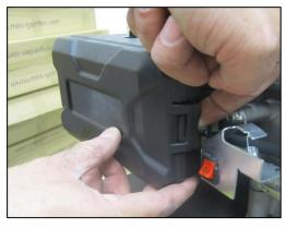
STEP 2: Lift tab to remove Air Filter Cover.
