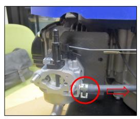
**STEP 7:** Use pliers to squeeze and loosen the Pinch Clamp on the Gas Line. Then gently pull off the Gas Line.
