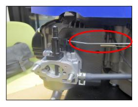
**STEP 5:** Locate the gas throttle wire and tension spring.
