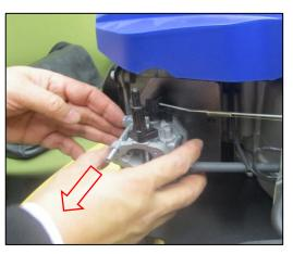
**STEP 8:** Grab onto the Carburetor by hand to remove it. Follow above steps in reverse to install the new Carburetor.
