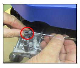
**STEP 6**: Unhook the gas throttle wire and tension spring.
