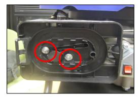
STEP 4: Unscrew the 2 nuts from inside the Air Filter box using an M10 wrench. Remove the Air Filter box.
