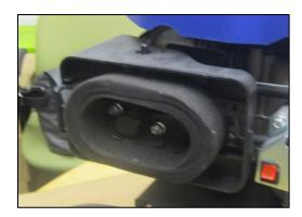
STEP 3: Remove the Air filter
