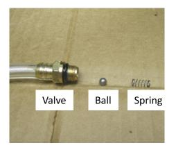
**STEP 3:** Unscrew and remove the Detergent Injector Valve. Disconnect the tube from the Valve and insert the new Valve. Replace the new Detergent Injector by placing the Spring and Ball into the injector as shown in this image. The Ball should be held in place with the Spring.
