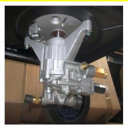
**STEP 2:** Use a wrench to remove the Detergent Injector Valve found underneath the Pump assembly. Be careful not to lose the small ball and spring located inside the Detergent Injector.
