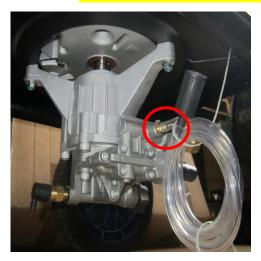
**STEP 1:** Remove the detergent tube to access to the detergent injector.
