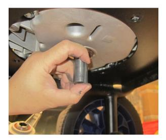
**STEP 2:** Verify that the Lock Key has remained in place on the Motor Drive Shaft Keyseat. If the lock key is inside the pump keyway, remove and place on the Drive Shaft Keyseat.
