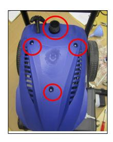
STEP 1: Remove the three bolts from the Top Cover, which is where the Recoil Starter Assembly is located. Keep the bolts.
