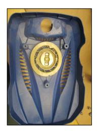
**STEP 2:** Remove Recoil Starter Assembly and assemble the new one by placing it back into position and fastening the three bolts and gas cap.
