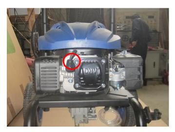
**STEP 1:** Clean out the area around the spark plug before removal to prevent impurities from falling inside the engine.
