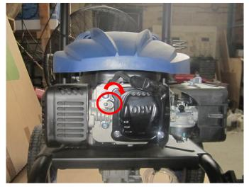
**STEP 5:** Use the spark plug wrench and continue tightening turning CLOCKWISE until it stops. Do not over-tighten or you may crack the porcelain. If using a torque wrench, torque between 12 to 15 lbs. See Figure 3.
