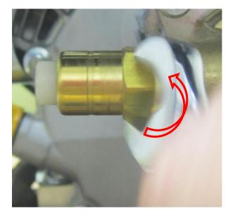
**STEP 2:** Use a wrench to remove the Thermal Relief Valve by turning it counter-clockwise.
