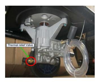
**STEP 1:** Remove the black cap from the thermal relief Valve, simply slide it off by hand.
