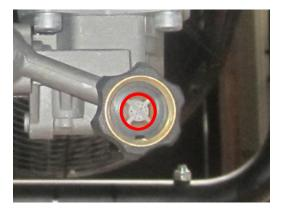
STEP 1: Using needle nose pliers, grab a firm hold of the plastic Water Filter found inside the Water Inlet and pull on the Water Filter to remove.
