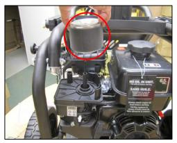
**STEP 2**: Remove the Air Filter. The Carburetor is located underneath.
