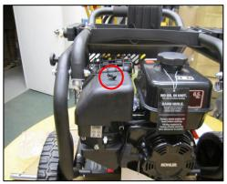
**STEP 1:** Unscrew the Wing Nut securing the Air Filter Cover. Remove Cover.
