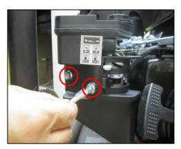
**STEP 3:** Using a metric #10 wrench, remove the two nuts that hold the Carburetor Cover, and loosen cover, but do not detach.
