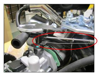
**STEP 8:** Unhook the gas throttle wire and tension spring
