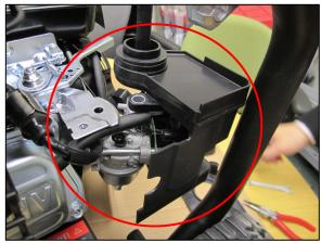
**STEP 5:**Remove the Carburetor Cover. Use the wrench to pry and slide out the Cover.
