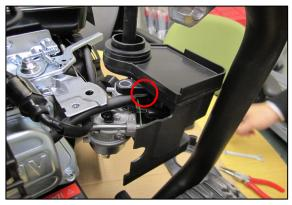
**STEP 4**: Disconnect the Air Filter rubber hose from the back of the cover.
