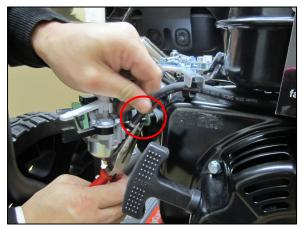
**STEP 7**:Use pliers to loosen the Pinch Clamp on the Gas Line and detach the Gas line from the Carburetor by pulling it off while squeezing the Pinch Clamp.
