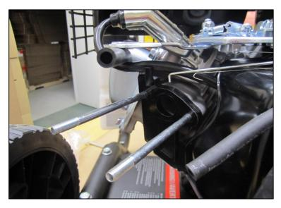
**STEP 11**: You have successfully removed the Carburetor. Follow above steps, in reverse, and carefully to install the new Carburetor.
