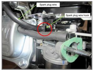
**STEP 6:** Make sure the Spark Plug Wire is seated in the Spark Plug Wire Hook.
