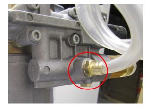
**STEP 2:** Use a wrench to remove the Detergent Injector Valve found underneath the pump assembly. (Above photo taken from below). Careful not to lose the small ball that is held by the Detergent Injector Valve.
