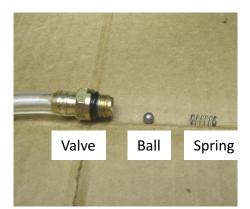
**STEP 3:** Unscrew and remove the Detergent Injector valve. Disconnect the tube from the valve to insert the new valve. Replace the new Detergent Injector by placing the Ball and Spring into the Injector as shown. The ball should be held in position by the Spring. Reattach valve to machine.
