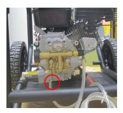
**STEP 1:** Locate the Detergent Injector
