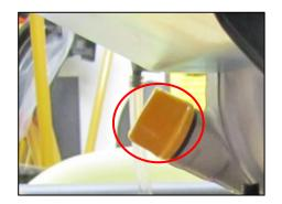
**STEP 5**: Remove the dipstick. Use a funnel to fill the crankcase with new oil up to the filler neck. Oil level should be at top of indicator on dipstick. Reinstall Oil fill plug/dipstick and tighten securely.
