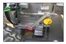
**STEP 4**: Using a wrench, remove the oil drain plug and allow oil to drain. After drainage, return the oil drain plug and tighten.
