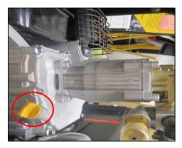
**STEP 2:** Use a rag to clean around oil fill area. Prepare an oil pan to catch the oil. Layer the work area with newspaper or cardboard to catch any spills.
