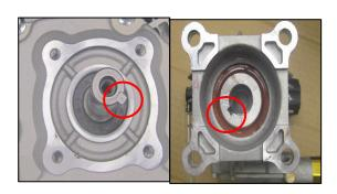
**STEP 3**: When sliding the new pump on the drive shaft, align the pump hub keyway with the drive shaft keyway. Assemble the four bolts using the M13 wrench, **but do not tighten.**
