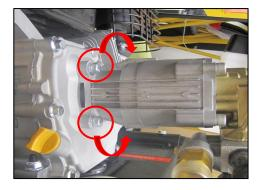
**STEP 1**: Using the M13 wrench, remove the 4 bolts that holds the pump assembly.
