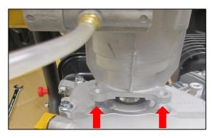
**STEP 2:** Firmly hold the pump with both hands and pull to slide the pump off the drive shaft.
