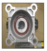
**STEP 4:** <u>IMPORTANT:</u> Before tightening the bolts, rotate the engine by gently pulling on the starter cord once. Screw on the bolts in a star pattern to evenly distribute the stress. Tighten each bolt partially, then move to the next one. Continue in a star pattern until they are all tight.
