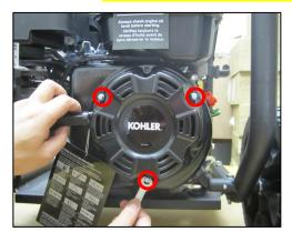
**STEP 1**: Using the wrench, remove the three bolts that hold the Recoil Starter. Save the bolts.
