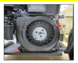
**STEP 2**: Grab the Recoil Starter with both hand and remove. Insert new Recoil Starter and fasten with M8 wrench.
