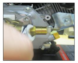
**STEP 2:**Use a wrench to remove the Thermal Relief Valve by turning it counterclockwise. Replace with new Thermal Relief Valve and re-attach the Rubber Cap.
