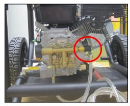
**STEP 1**: Remove the rubber cap from the Thermal Relief Valve and slide it off.
