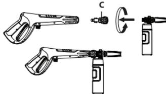
1. Attach the adaptor 2 (C) onto the plastic spray gun.
