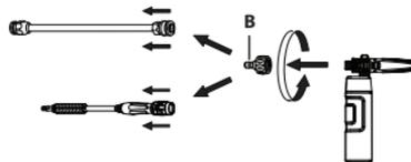
1. Attach the adaptor 1 (B) onto the quick-connect wand.
