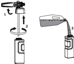
1. Rotate the foam blaster's spray head from vertical position to horizontal position.
