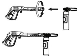
1. Attach the foam blaster onto the spray gun.
